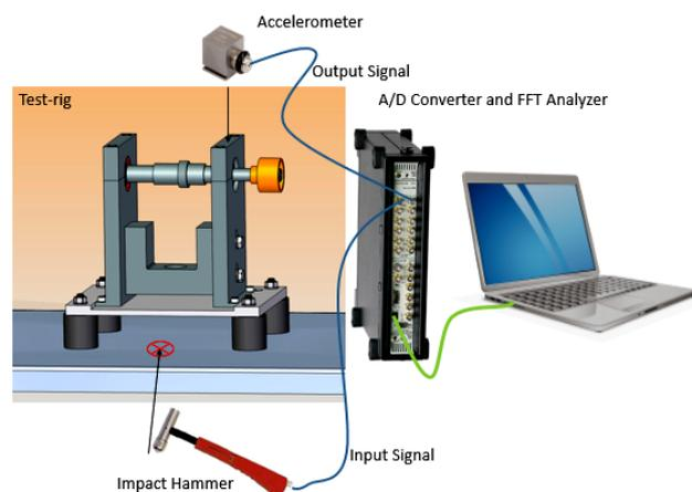
Figure 5. Experimental setup diagram
