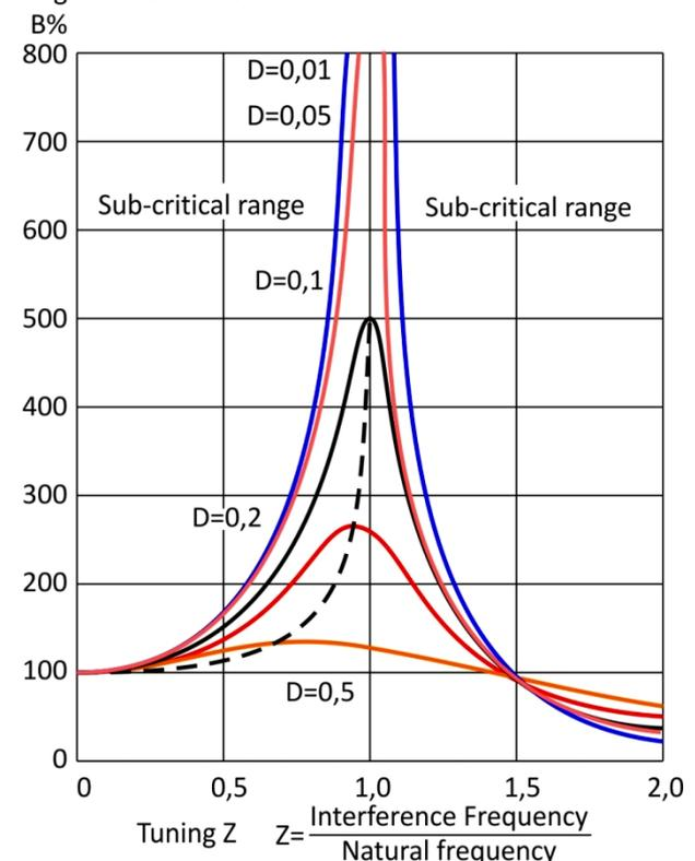
**Figure 2.** Steady state variation of amplitude with frequency and damping of a driven simple harmonic oscillator
