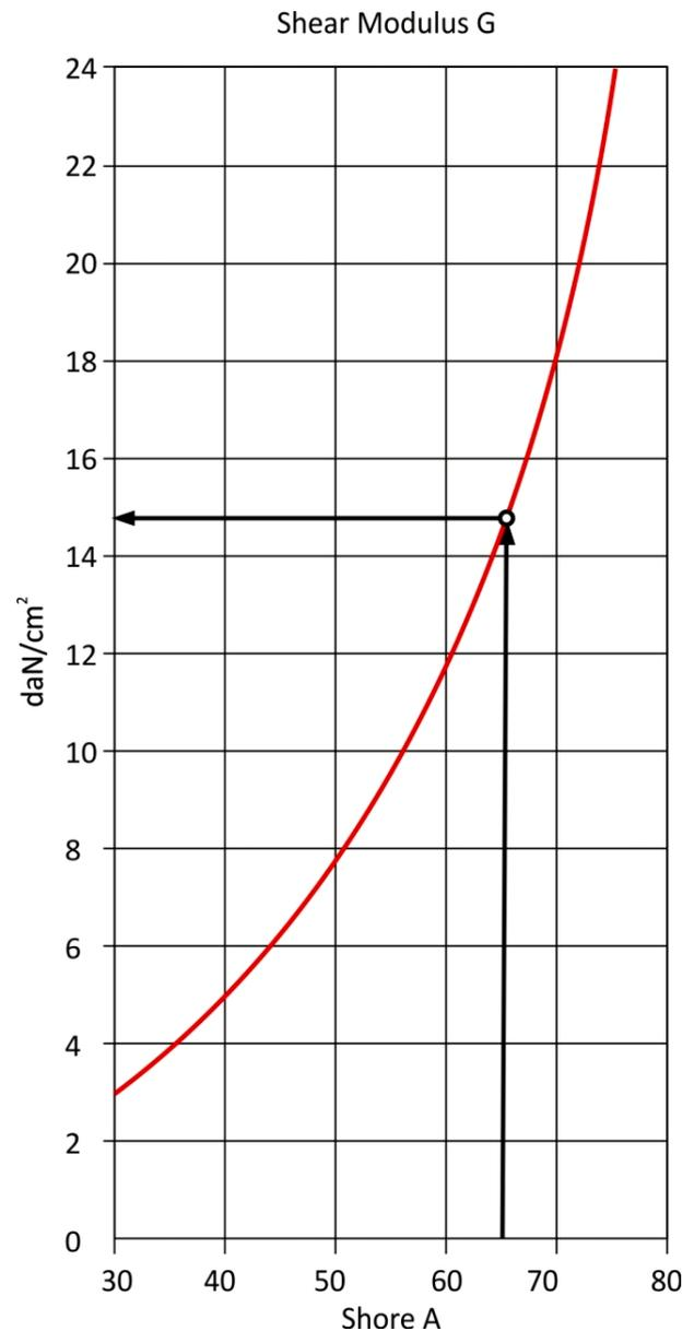
Figure 1. Relationship between hardness and shear modulus
