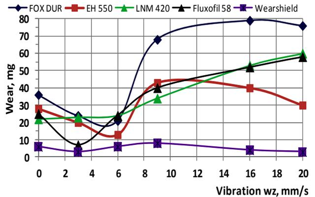
**Figure 9.** Wear vs. vertical vibration speed component  $w_z$
