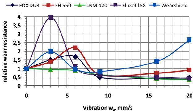
Figure 11. Relative wear-resistance vs. vertical vibration speed component  $w_z$
