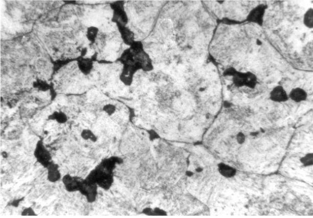
Figure 4. Microstructure of coating LNM 420; 500 ×
