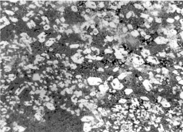
Figure 6. Microstructure of coating Wearshield 70; 500 ×
