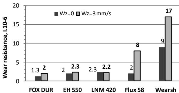
Figure 12. Diagram of coatings wear-resistance without and with vibration  $w_z = 3$  mm/s
