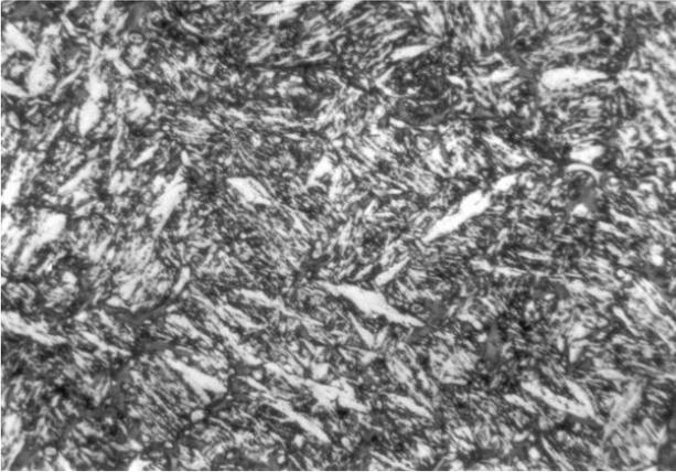
Figure 5. Microstructure of coating Fluxofil 58; 500 ×
