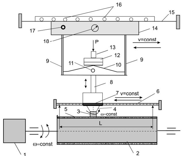
Figure 7. Functional scheme of the device for the study of abrasive wear under the vertical vibrations in the pin-on-cylinder device
