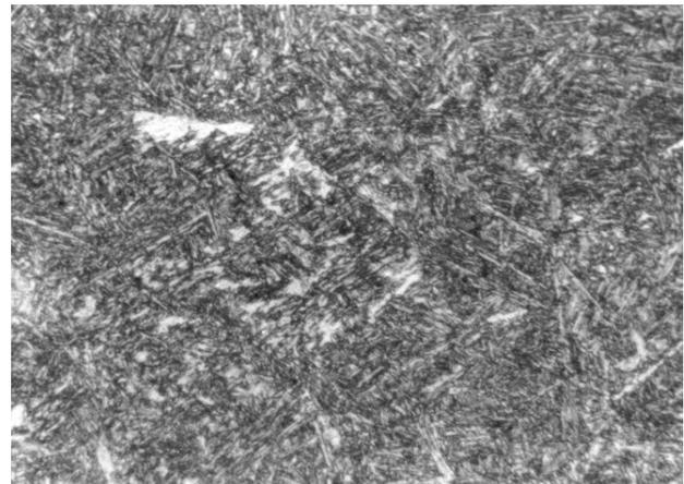
**Figure 2.** Microstructure of coating FOX DUR 350; 500  $\times$
