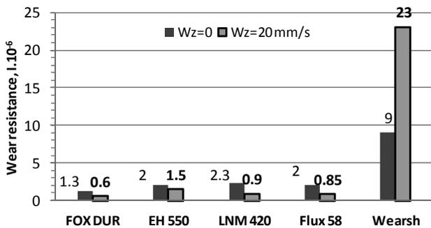
Figure 13. Diagram of coatings wear-resistance without and with vibration  $w_z = 20$  mm/s
