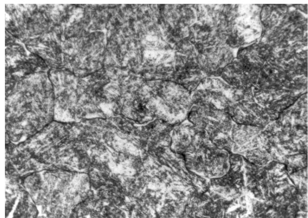
**Figure 3.** Microstructure of coating EH 550; 500  $\times$
