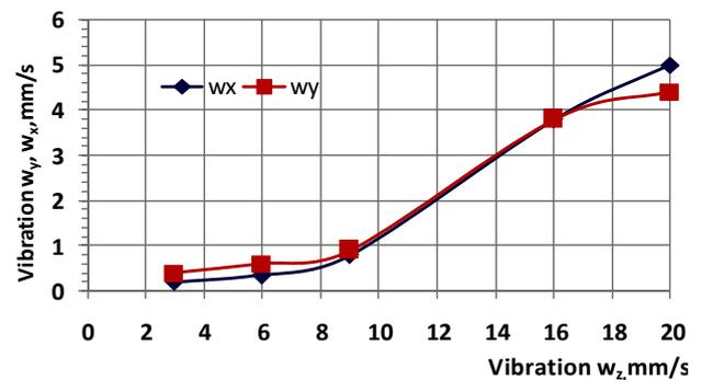
**Figure 10.** Relationship between vibration speed components  $w_z$ ,  $w_x$  and  $w_y$
