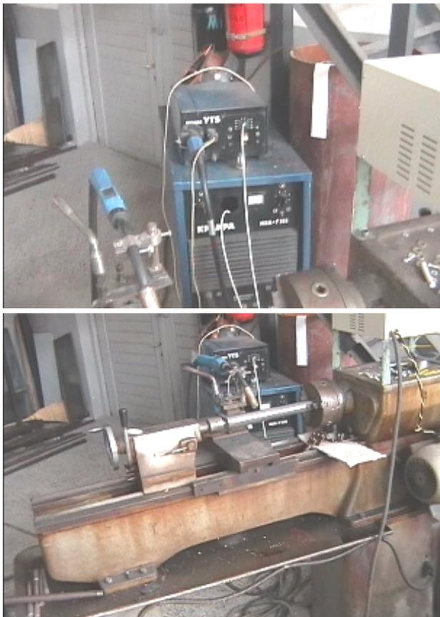
**Figure 1.** Device for cladded coatings arc deposition
