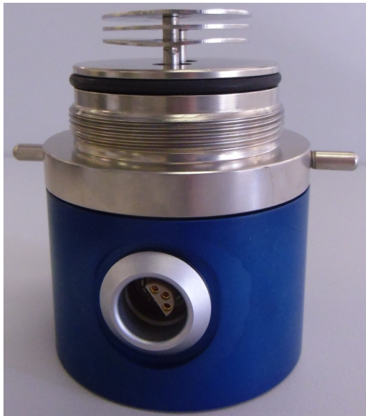
Figure 1. Sensor with triple plate design
