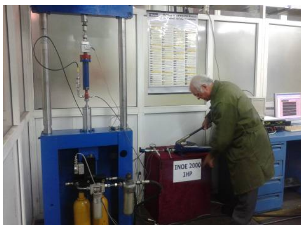
Figure 4. Creating pressure with hand pump
