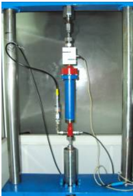
Figure 9. Experimental device for piston seal
