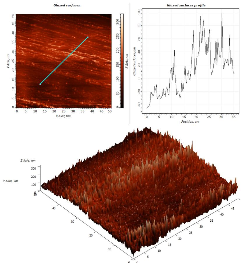
**Figure 5.** 3D topography and roughness profile of glazed surface of the lithium disilicate glass ceramic
