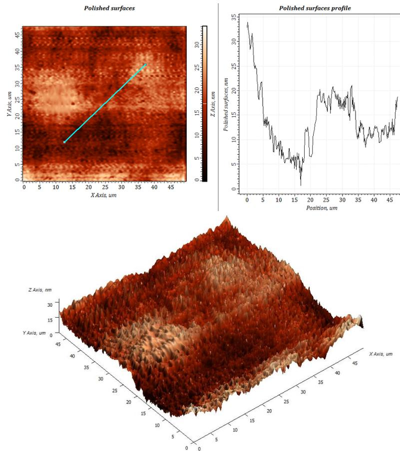
**Figure 4.** 3D topography and roughness profile of polished surface of the lithium disilicate glass ceramic
