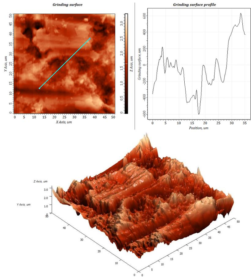
**Figure 6.** 3D topography and roughness profile of grinding surface of the lithium disilicate glass ceramic
