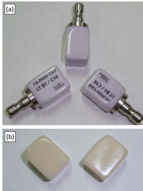
**Figure 1.** Lithium disilicate blocks (IPS e.max CAD): (a) partially crystallized blocks and (b) final state of crystallized blocks
