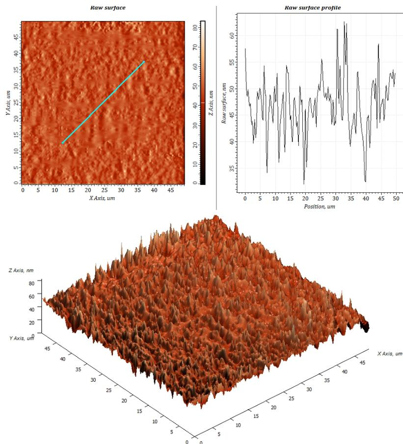
**Figure 7.** 3D topography and roughness profile of raw surface of the lithium disilicate glass ceramic
