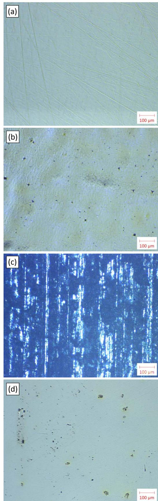
**Figure 2.** Contact surfaces of lithium disilicate glass ceramic (IPS e.max CAD) treated with different finishing procedure: (a) polished surface, (b) glazed surface, (c) ground surface, and (d) contact surface of raw materials
