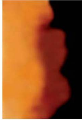
Fig. 1. Atomic Force Microscopy (AFM) picture of a monolayer of graphene, [1] (the black area is the silicon substrate, the dark orange is a mono layer of graphene with thickness of~ 0.5 nm, the bright orange part contains a few layers with thickness of~ 2 nm)
