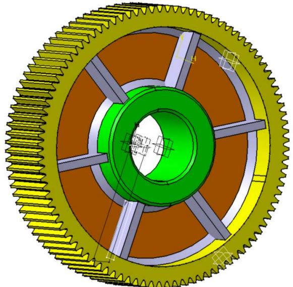
Figure 5: Cylindrical gear made by welding
