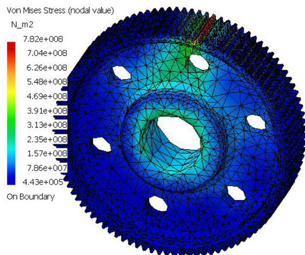
Figure 7: Stress values of loaded gear model calculated in structural analysis
