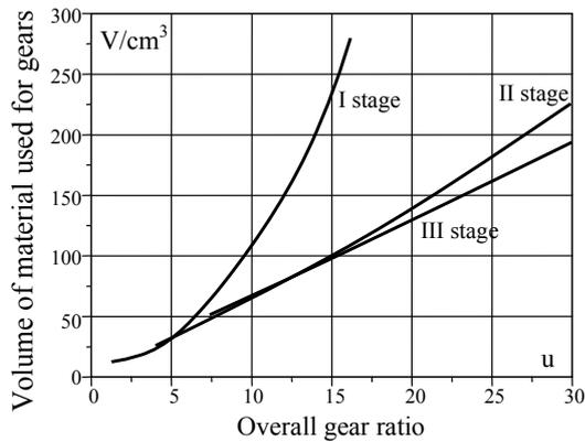
Figure. 1: The relation between the volume of gear train and overall gear ratio.
