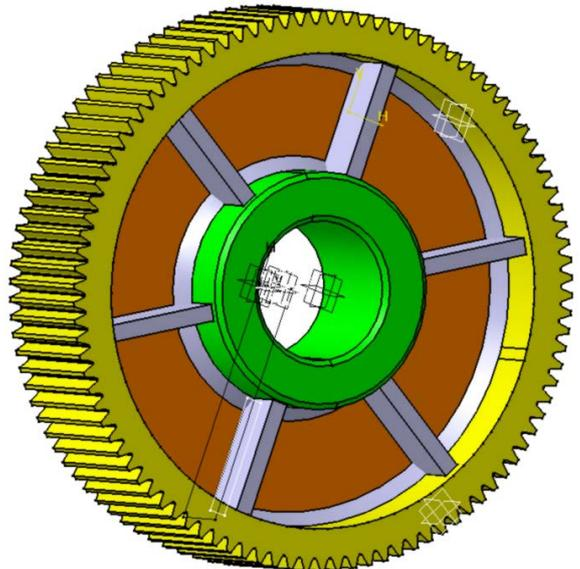
Figure 5: Cylindrical gear made by welding
