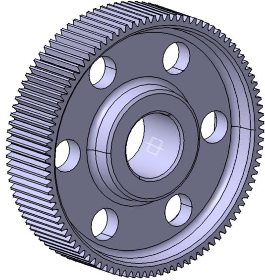
Figure 4: Press made model of cylindrical gear
