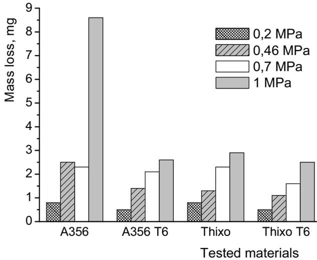
**Figure 5:** Mass losses of tested materials for different specific loads.
