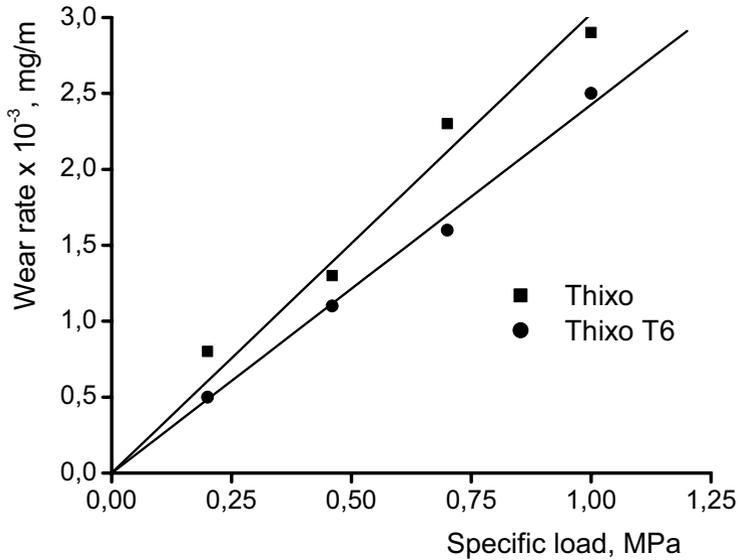
**Figure 6:** Wear rate vs. specific load for thixocasted specimens.
