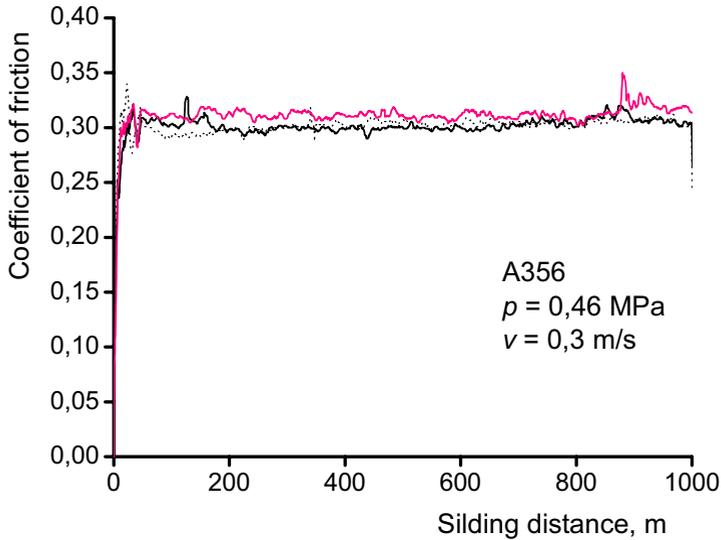
**Figure 3:** Diagram showing reproducibility of wear tests (Coefficient of friction vs. sliding distance).
