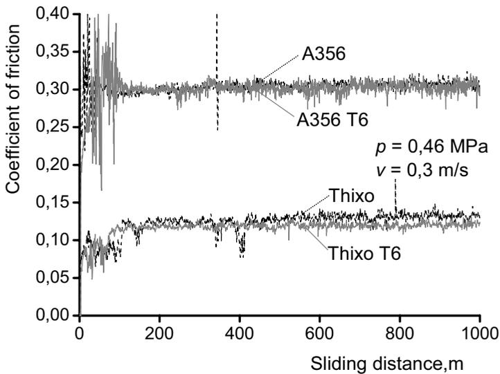
**Figure 4:** Coefficient of friction vs. sliding distance for  $p = 0,46 \text{ MPa}$  and  $v = 0,3 \text{ m/s}$ .
