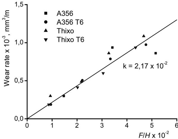
**Figure 7:** Wear coefficient for tested materials.
