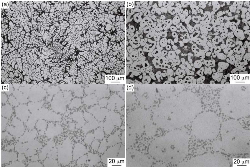
**Figure 1:** Microstructure of tested materials (a) A356, (b) A356 T6, (c) Thixo and (d) Thixo T6.
