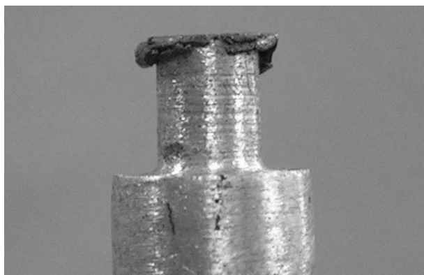
Fig. 3. Plastic deformation of pin KA356 at 1.46 MPa
