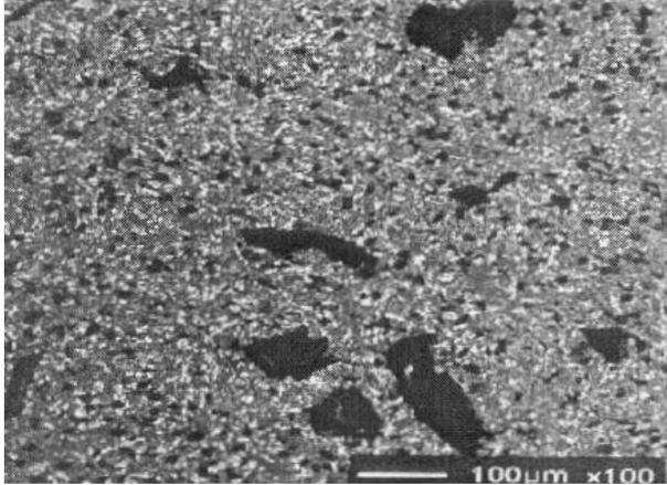
**Figure 1.** Hybrid composite containing 10 % SiC and 4 % graphite particles [1]
