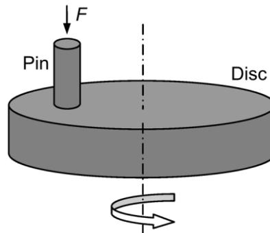
Figure 2. Schematic diagram of the pin-on-disc tribometer
