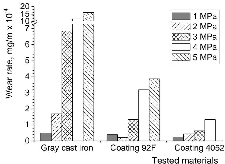
Figure 3. Wear rates of the tested materials for different specific loads
