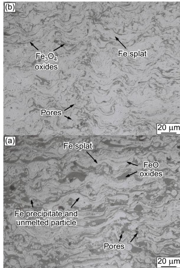
Figure 1. OM cross-section micrograph of: (a) coating 92F and (b) coating 4052
