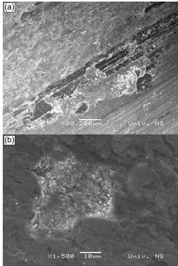
Figure 5. SEM micrographs of the pins worn surfaces: (a) coating 92F at 2 MPa and (b) coating 4052 at 4 MPa
