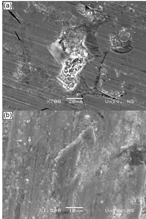
Figure 4. SEM micrographs of the pins worn surfaces: (a) gray cast iron at 2 MPa and (b) gray cast iron at 5 MPa
