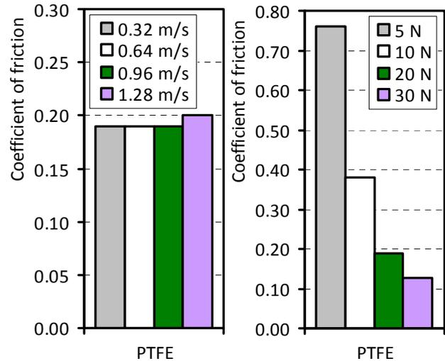
**Figure 3.** Sensitivity of PTFE coefficient of friction to the sliding speed (for 20 N load) and applied load (for 0.32 m/s speed) (adopted from [8])
