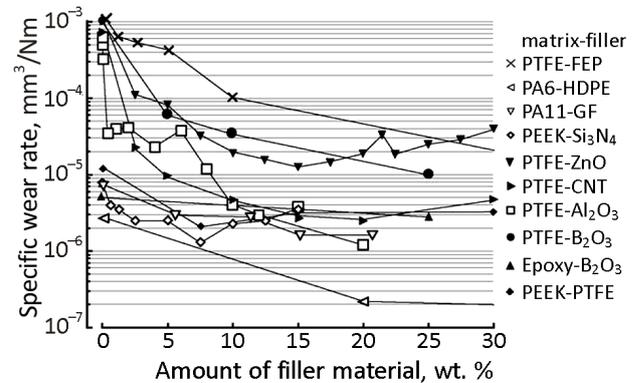
**Figure 11.** Specific wear rate vs. wt. % of filler material for various polymer composites (FEP – fluorinated ethylene propylene; PA6 – polyamide 6; HDPE – high-density polyethylene; PA11 – polyamide 11; GF – glass fibre; PEEK – polyether ether ketone; CNT – carbon nanotube)
