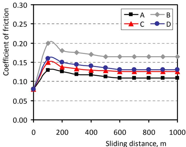
**Figure 2.** Frictional behaviour of PTFE and PTFE composites (adopted from [7])
