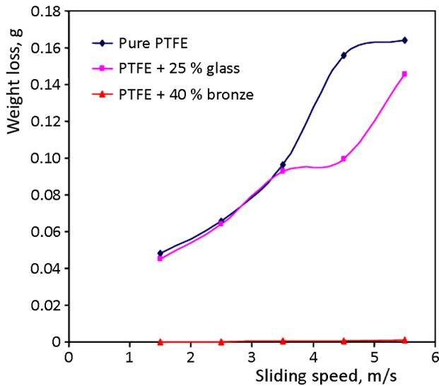
**Figure 4.** Weight loss vs. sliding speed at constant applied load of 60 N and sliding distance of 1500 m
