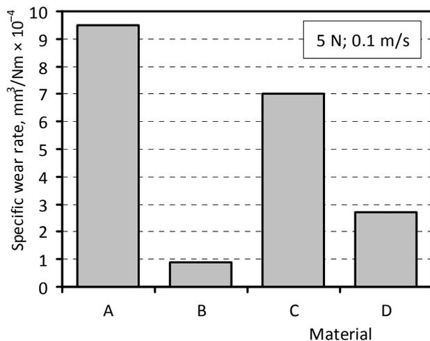
**Figure 1.** Average specific wear rate of PTFE and PTFE composites (adopted from [7])
