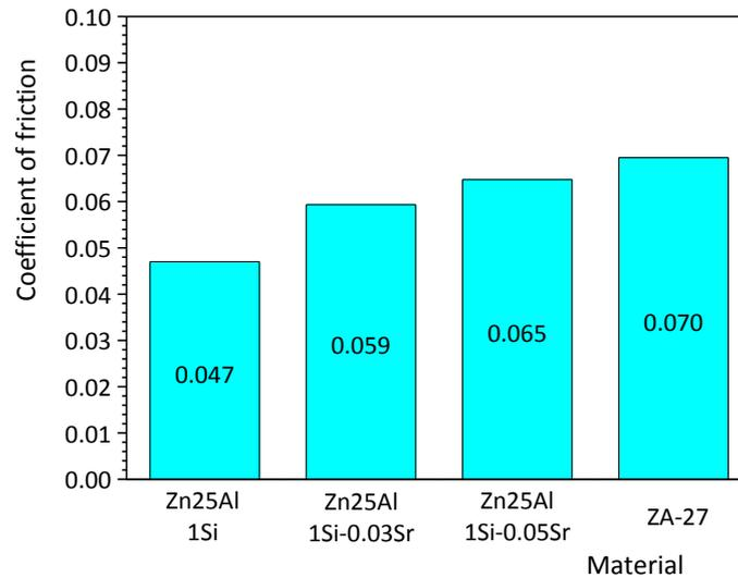
**Fig. 3. Steady-state averaged values of the coefficient of friction**
