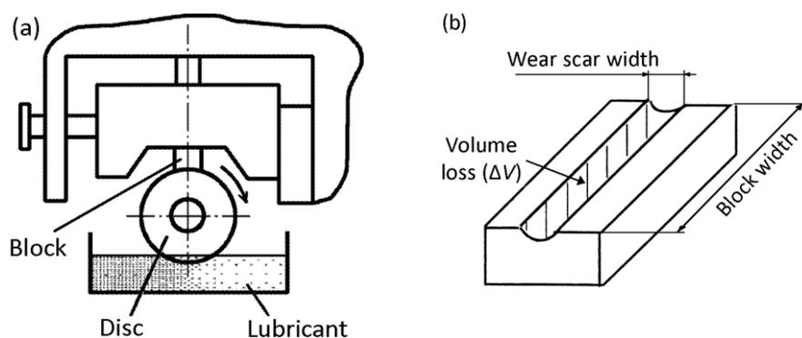
**Fig. 2. Tribological testing: (a) schematic diagram of the block-on-disc tribometer and (b) block wear scar measurements**
