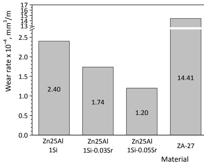
**Fig. 4. Total wear rates for the tested materials**
