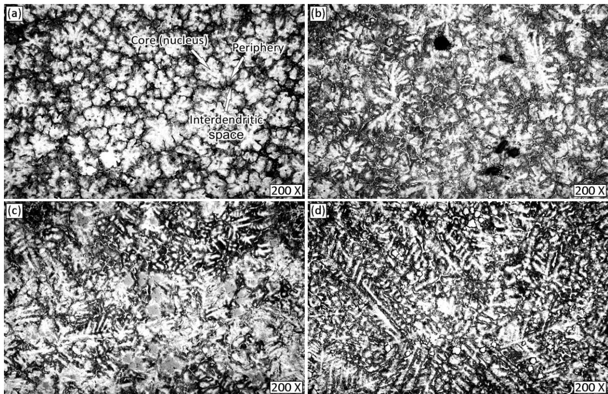
**Fig. 1. Microstructures of tested materials: (a) ZA-27 alloy, (b) Zn25Al1Si alloy, (c) Zn25Al1Si-0.03Sr alloy and (d) Zn25Al1Si-0.05Sr alloy**
