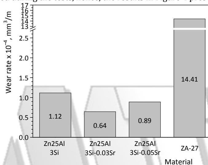
**Figure 4. Total wear rates for the tested materials**
