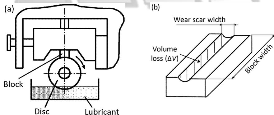
**Figure 2. Tribological testing: (a) schematic diagram of the block-on-disc tribometer and (b) block wear scar measurements**
