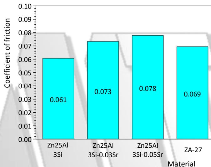
**Figure 3. Steady-state averaged values of the coefficient of friction**
