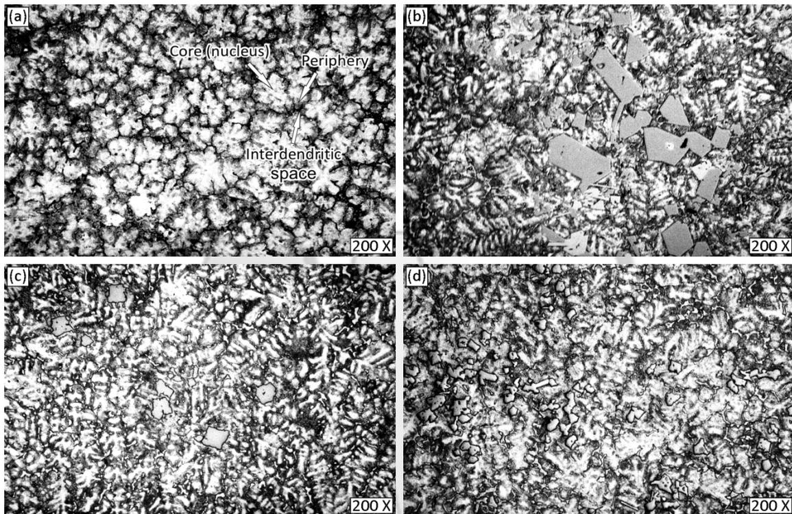
**Figure 1. Microstructures of tested materials: (a) ZA-27 alloy, (b) Zn25Al3Si alloy, (c) Zn25Al3Si-0.03Sr alloy and (d) Zn25Al1Si-0.05Sr alloy**
