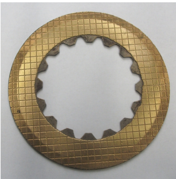
Figure 5. Wear track (lighter circular ring) on sample Cu-4Sn after 300 abrasion cycles (approx. 71.8 m)
