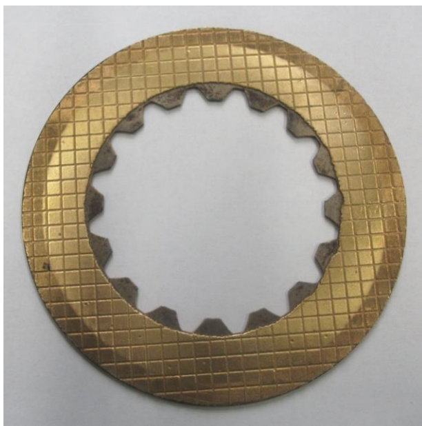
Fig. 5. Wear track (lighter circular ring) on sample Cu-4Sn after 300 abrasion cycles (approx. 71.8 m).
